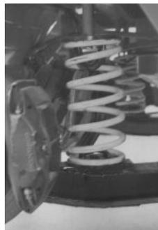
The front wheel springs have screw jacks that extend up to the engine compartment, but because the hood must be opened to reach them, they're rarely adjusted during a race. The rear screw jacks protrude through the rear-window glass, however, so they're easily accessible at all times.
